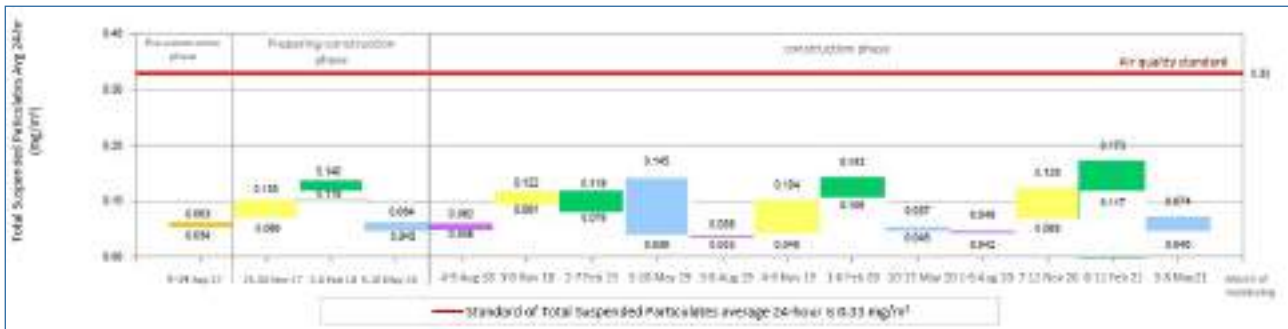
Photo depicting the result of TSP 24-hours monitoring nearby construction project
