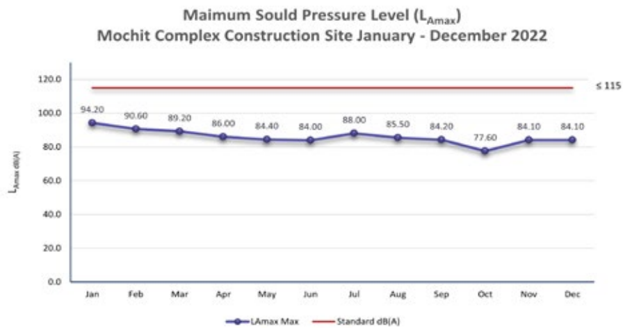
Result of maximum noise level monitoring results within the area of the Mochit Complex project, during the construction phase between January - December 2022.
